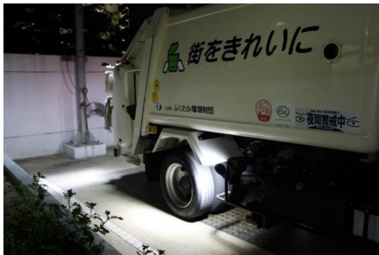
路肩灯 Lighting curbs
